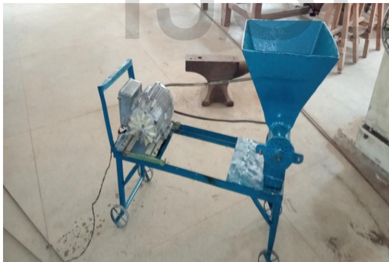
Figure 4: Shows the Pelletizing Machine Developed.
